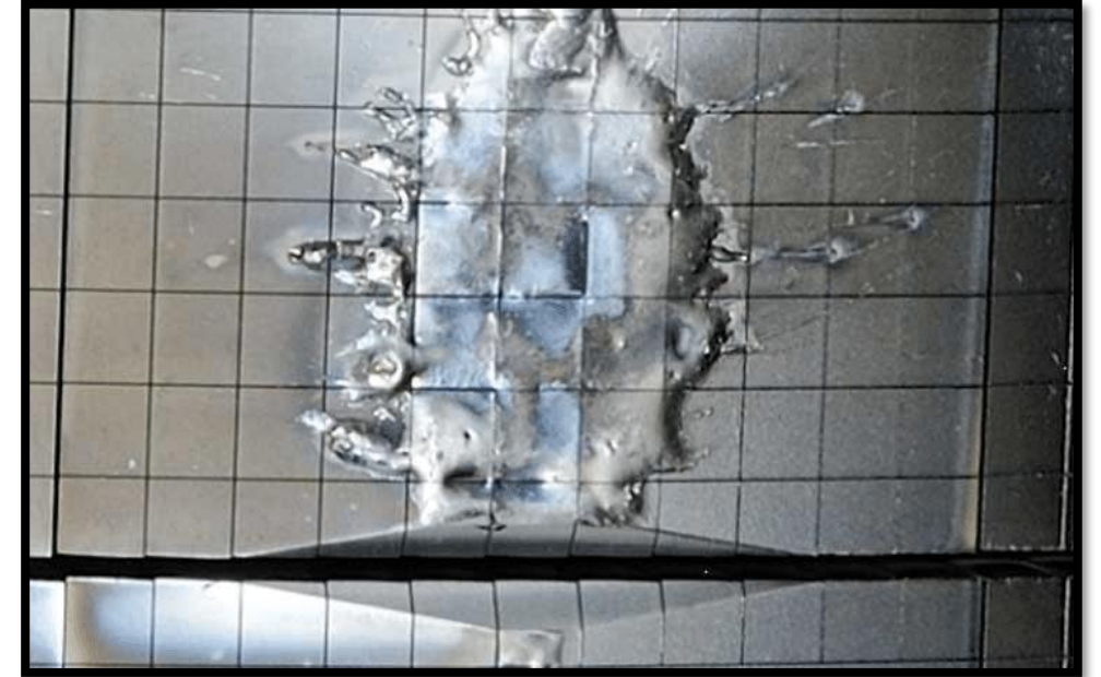
FIG. 2. Melting of a Beryllium tile in JET tokamak due to runaway electron
